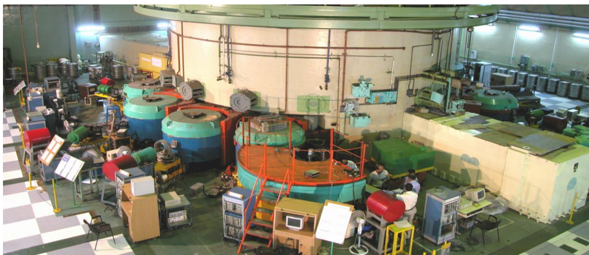
Fig. 2. Panoramic view of the neutron instruments at Dhruva. The instruments seen are, from left, triple axis spectrometer, polarisation analysis spectrometer, single crystal diffractometer, multi-position sensitive detector (PSD) based powder diffractometer, on the four tangential beamtubes, a single PSD based powder diffractometer at the end of a through-tube and filter detector spectrometer at the extreme right. The yellow coloured block is basically the shield of the instrument developed by the university researcher under UGC-DAE CSR. The hi-Q diffractometer and quasielastic spectrometer are on the opposite side and not seen in the photo. The guide tube laboratory is on the left of the reactor hall, the shielding of the guide is seen.
